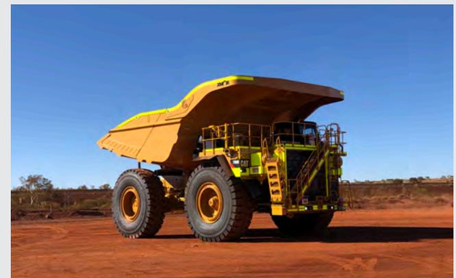
**First class dumping performance** - Floor and tail shape, as well as flared sidewalls result in load shedding that reduces contact pressure on floor, whilst also ensuring no choking as the material exits the tray. This enables the material to clear the windrow at the dump - avoiding tail dragging and dozer cleanup.
